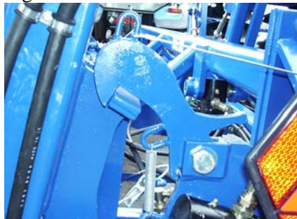
Transport lock on the packer roller
